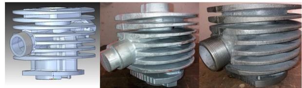
Figure 4: CAD model, 3D-printed casting mould and casted cylinder [6]
