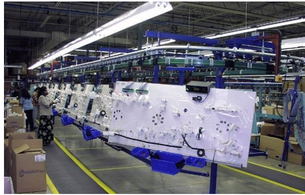
Figure 2: The most widely used open station paced conveyors are used in wire harness assembly, where the operators are working at tables that moving in every cycle of the production [12].
