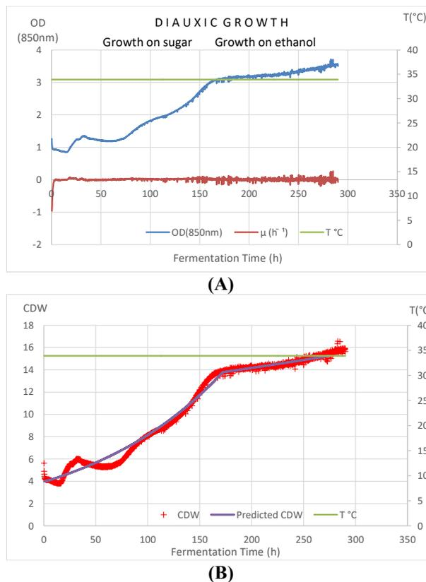
Figure 1. The measured parameters (temperature,  $\mu$ , OD<sub>850</sub>) and calculated data (CDW from OD<sub>850</sub>) along with the data of the predicted (i.e. fitted) model. (A) green line: temperature; blue line: measured turbidity at 850nm; brown line: measured specific growth rate. (B) green line: temperature; red crosses: calculated cell dry weight from the measured turbidity at 850nm; purple line: fitted model-based prediction for CDW.
