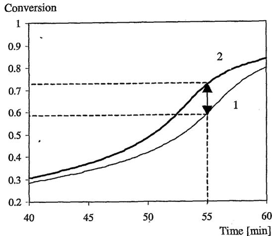
Fig. 7 The influence of temperature increase on monomer conversion; 1 - initial conversion; 2 - disturbed conversion caused by temperature change
