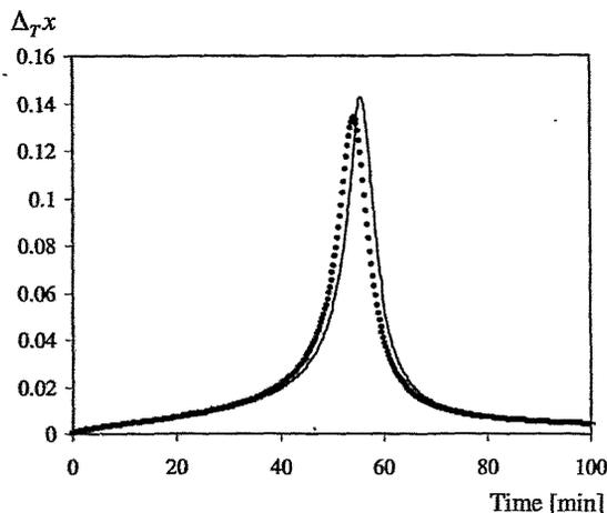
Fig. 6 The conversion variation caused by temperature increase; solid line - calculus based on sensitivity functions; dotted line - calculus based on model simulations
