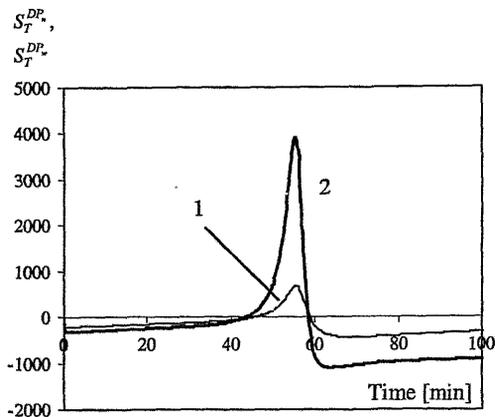
Fig. 5 The variation in time of sensitivity functions  $S_T^{DP_n}$  (1),  $S_T^{DP_w}$  (2)
