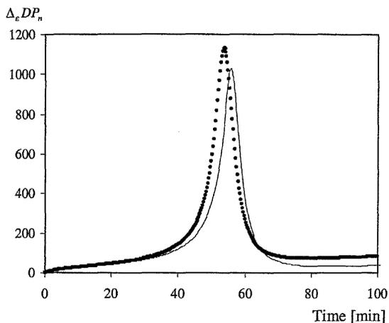
Fig.8 The variation of numerical average polymerization degree caused by  $\epsilon$  parameter change; solid line - calculus based on sensitivity functions; dotted line - calculus based on model simulations
