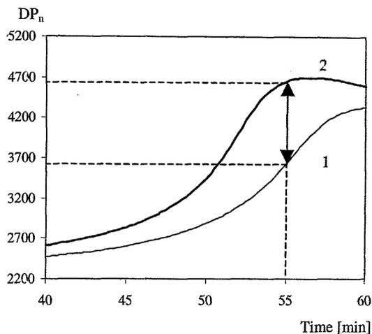
Fig.9 The influence of  $\epsilon$  parameter change on numerical average polymerization degree; 1 - initial  $DP_n$ ; 2 - disturbed  $DP_n$
