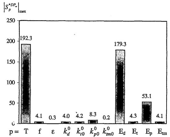
Fig.4 The histogram of maximum absolute values  $|S_p^{*DP_w}|_{max}$  showing the influence of parameters on gravimetric average polymerization degree
