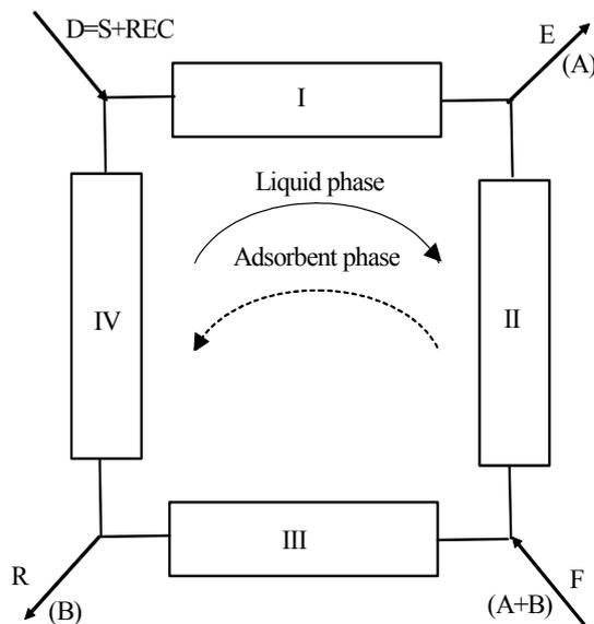
Fig. 2. Simulated Moving Bed (SMB)
