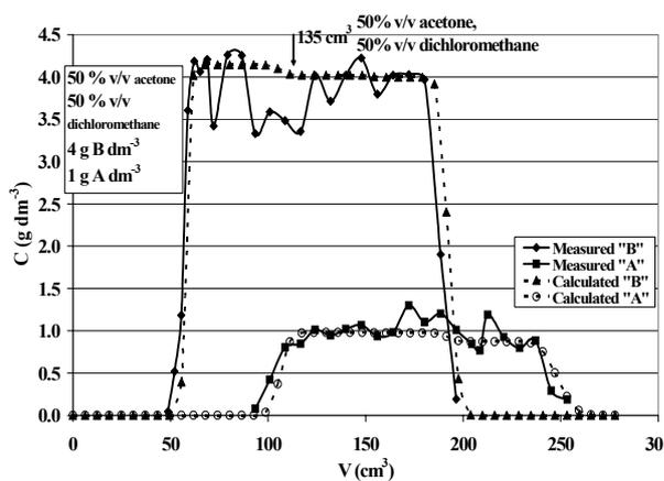
Fig. 5. Frontal adsorption-desorption measurement of steroids
