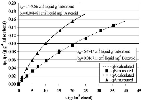
Fig. 4. Adsorption equilibria measurement of „A” and „B” components
