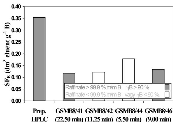
Fig. 12. Comparing the eluent consumption of steroid B in different measurements
