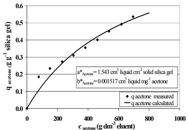
Fig. 3. Adsorption equilibria measurement of acetone
