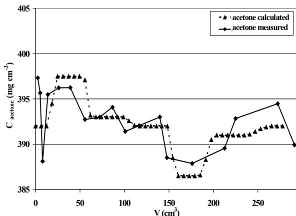
Fig. 6. Frontal adsorption-desorption measurement of acetone
