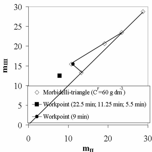
Fig. 8. The measurements points placed in the Morbidelli triangle at different switching times
