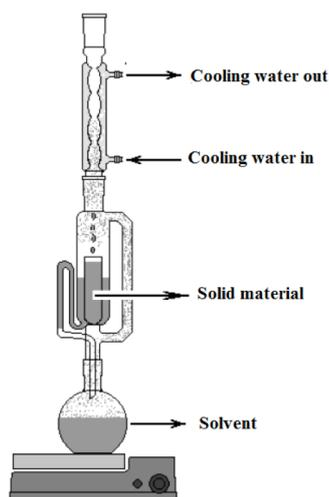
Figure 1: Soxhlet extractor [12]
