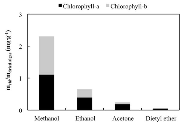
Figure 5: Efficiency of leaching using the various solvents
