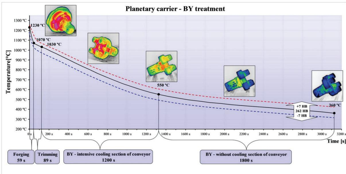
Figure 10: Cooling diagram of planetary carrier
