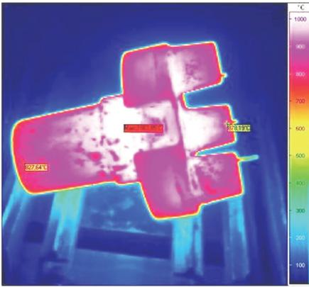
Figure 7: Photo taken by thermographic camera on start of intensive cooling stage. Emission factor: 0.95
