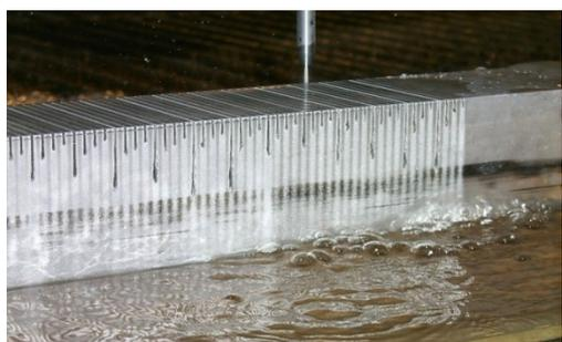
Figure 3: Kerfing tests in AlMgSi0,5 Aluminium Alloy
