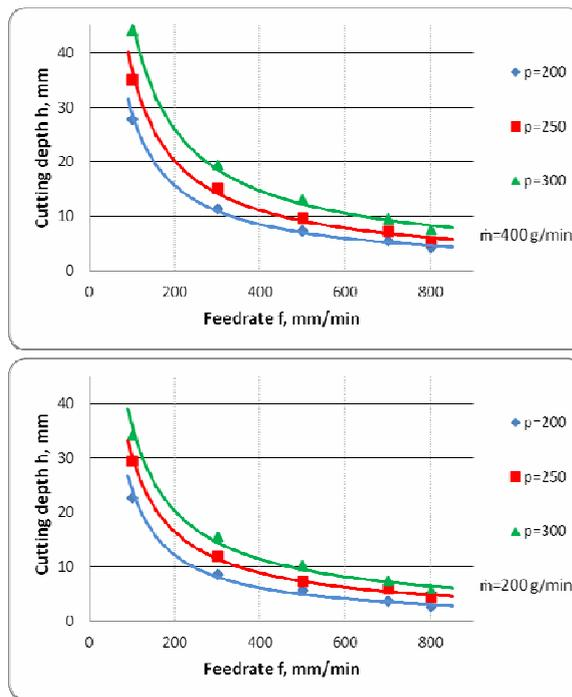
Figure 4: Effect of the feedrate on the depth of kerf at different pressures and abrasive mass flow rates, on AlMgSi0,5 aluminium alloy
