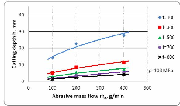
Figure 6: Effect of the abrasive mass flow rate on the depth of kerf at different feedrates and pressures, on AlMgSi0,5 aluminium alloy
