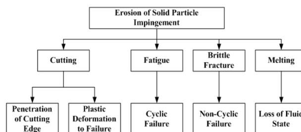
Figure 1: Material removal processes in course of solid particle erosion
