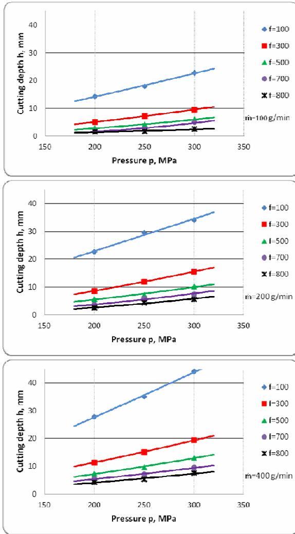
Figure 5: Effect of the pressure on the depth of kerf at different feedrates and abrasive mass flow rates, on AlMgSi0,5 aluminium alloy
