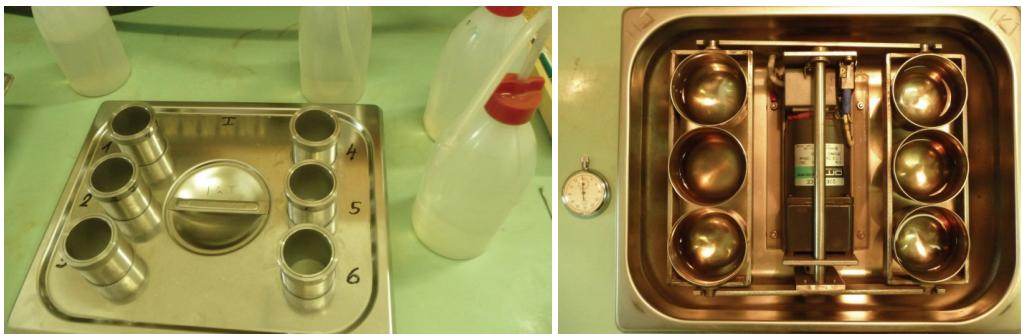
Figure 1: Wet sieving apparatus for aggregate stability measurement
