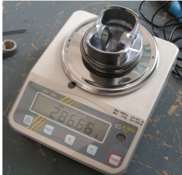
Figure 6: Measuring the piston mass
