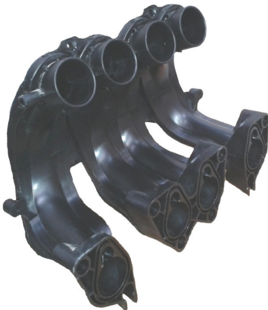
Figure 9: Lower intake system
