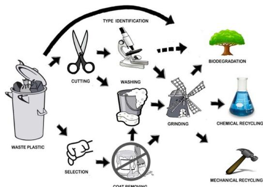
Figure 1: Pre-treatment and recycling of plastic wastes
