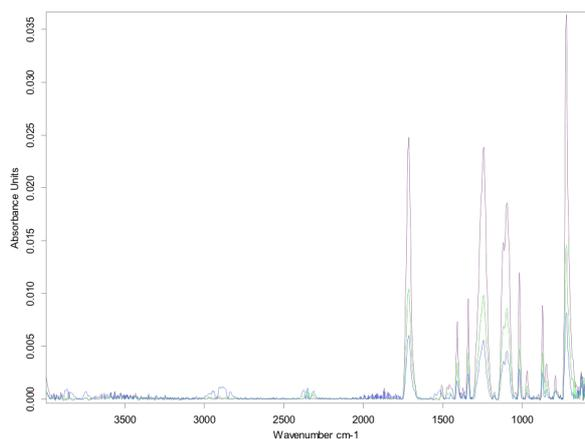
Figure 7: FT-IR spectra of PET sample in the 4000-600 cm<sup>-1</sup> wavenumber range (purple: potassium-hydroxide; green: citric acid; blue: without washing)
