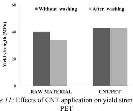
Figure 11: Effects of CNT application on yield strength of PET
