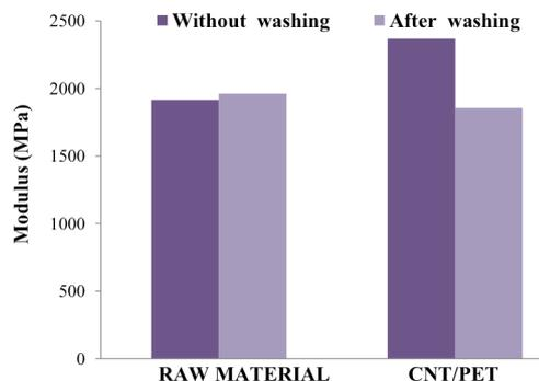
Figure 12: Effects of CNT application modulus of PET
