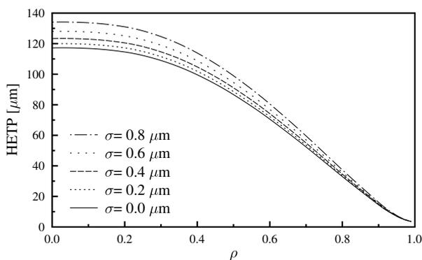
Figure 4: HETP of columns packed with 2.6  $\mu\text{m}$  core-shell particles
