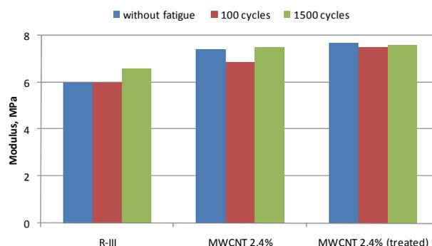
Figure 10: Effects of surface treatment on fatigue tensile properties of the composites (fatigue load: 10 N)
