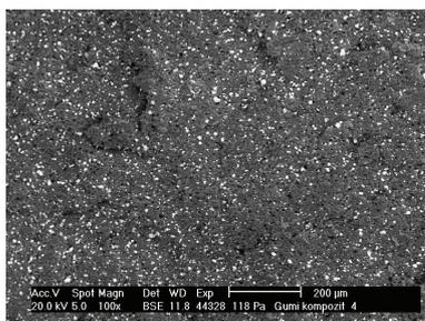
Figure 13: SEM graph of the broken surface of the pristine CNT containing rubber composite
