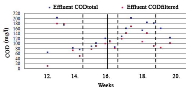
Figure 5: COD removal in the 50% CNT reactor
