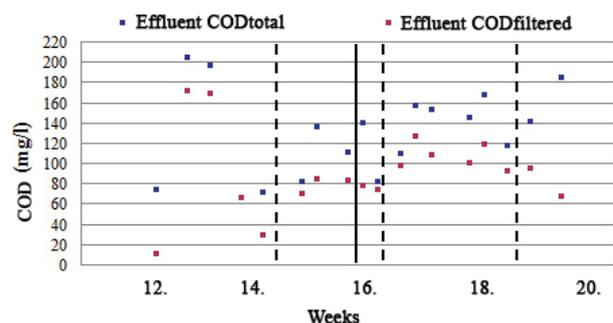
Figure 4: COD removal in the 100% HDPE reactor
