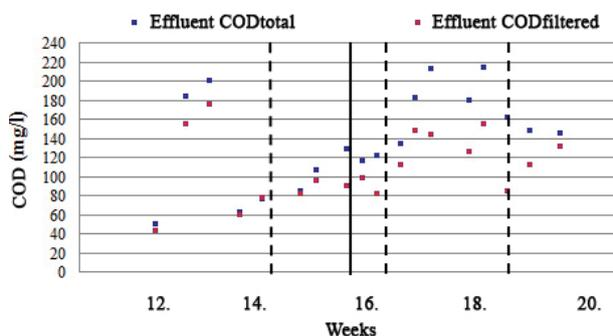
Figure 6: COD removal in the 75% CNT reactor
