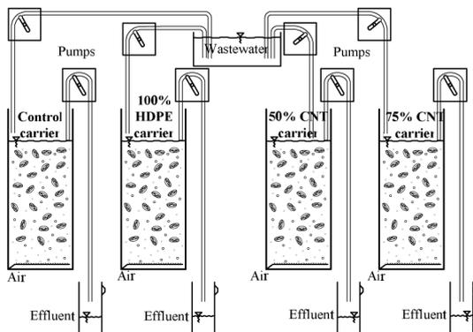
*Figure 1*: 4 parallel reactors
