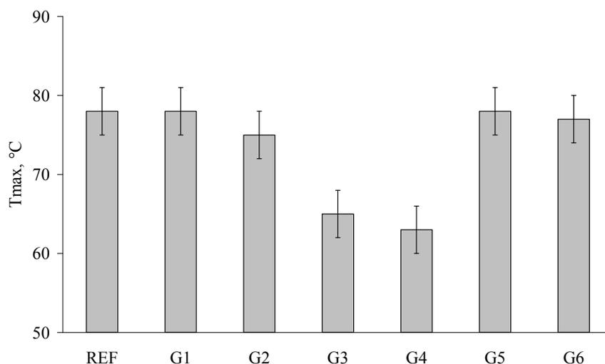
Figure 4: Antifriction properties of the experimental engine oils
