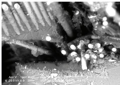
Figure 13: Fibre-matrix interaction in untreated chopped glass fibre mat reinforced polyester composites
