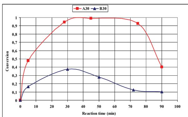
*Figure 4:* Hydrogen content of the outlet gas (A30: support „A”, C<sub>2</sub>H<sub>4</sub> flow rate 30 l/h; B30: support „B”, C<sub>2</sub>H<sub>4</sub> flow rate 30 l/h)
