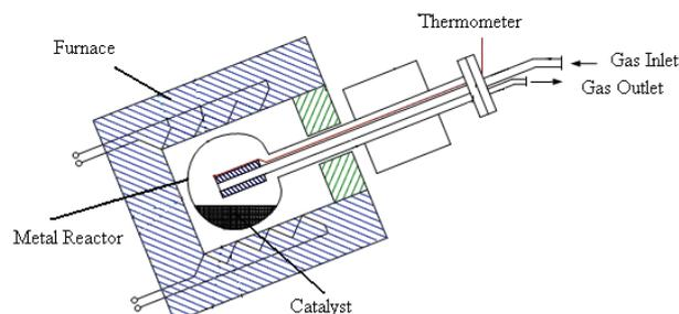
Figure 2: Scheme of pilot plant
