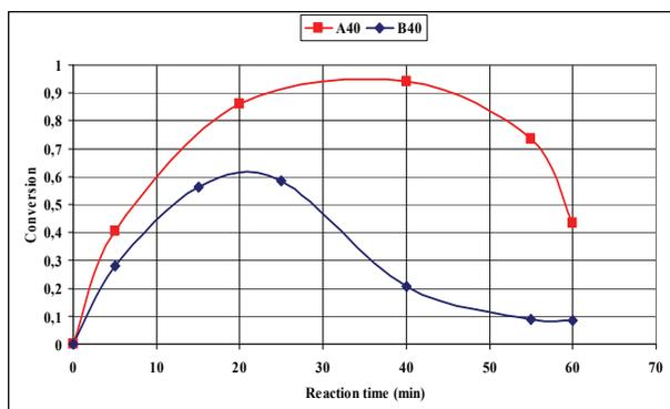
*Figure 3:* Hydrogen content of the outlet gas (A40: support „A”, C<sub>2</sub>H<sub>4</sub> flow rate 40 l/h; B40: support „B”, C<sub>2</sub>H<sub>4</sub> flow rate 40 l/h)
