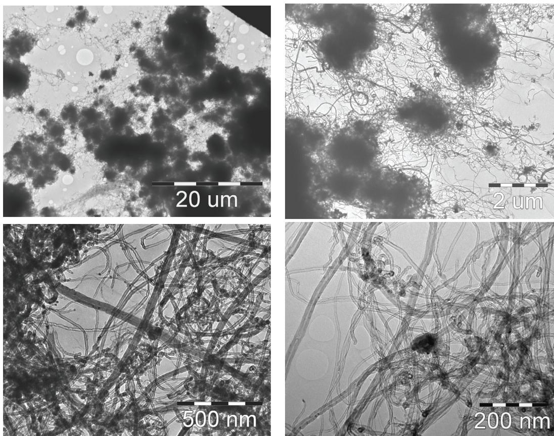
Figure 7: TEM images of MWCNTs produced by support „B”
