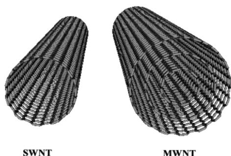
*Figure 1:* SWCNT and MWCNT
