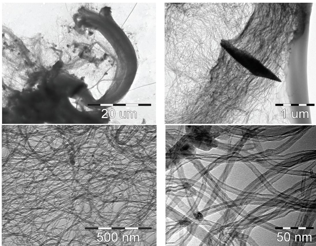
Figure 6: TEM images of MWCNTs produced by support „A”
