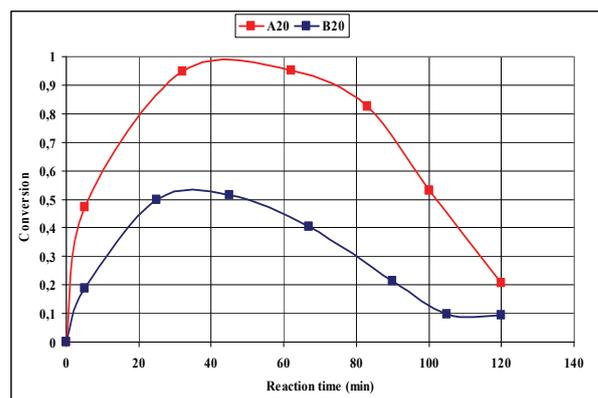
*Figure 5:* Hydrogen content of the outlet gas (A20: support „A”, C<sub>2</sub>H<sub>4</sub> flow rate 20 l/h; B20: support „B”, C<sub>2</sub>H<sub>4</sub> flow rate 20 l/h)
