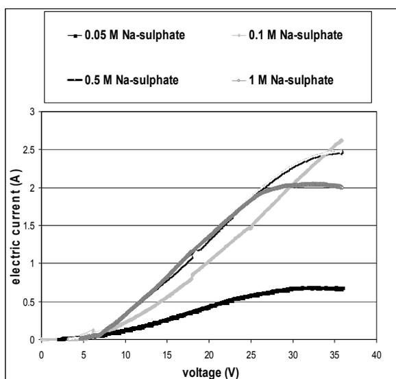
Figure 2: Potential drop as a function of electric current
