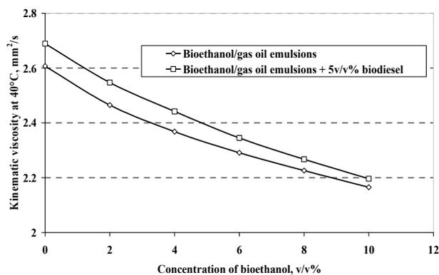
Figure 7: Change of kinematic viscosity of bioethanol/gas oil and/or biodiesel emulsions as a function bioethanol content
