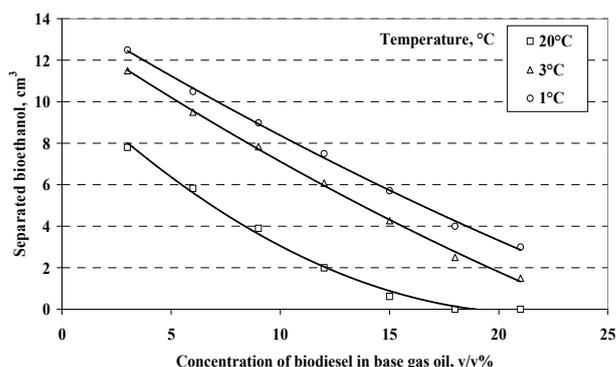
Figure 3: Stability of bioethanol/gas oil emulsions as a function of temperature (1% additive, 15 v/v% bioethanol)
