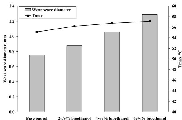
Figure 9: Change of lubricity of bioethanol/gas oil emulsions as a function of bioethanol content
