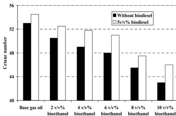
Figure 12: Change of cetane number of bioethanol/gas oil and/or biodiesel emulsions as a function of bioethanol content (biodiesel content of base gas oil: 5v/v%)
