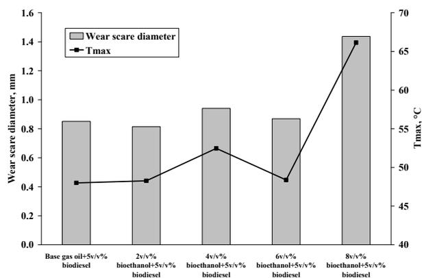
Figure 10: Change of lubricity of bioethanol/gas oil/biodiesel emulsions as a function of bioethanol content (biodiesel content of base gas oil: 5 v/v%)
