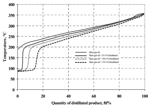
Figure 11: Change of the distillation properties of bioethanol/gas oil and/or biodiesel emulsions as a function of bioethanol content (biodiesel content of base gas oil: 5 v/v%)
