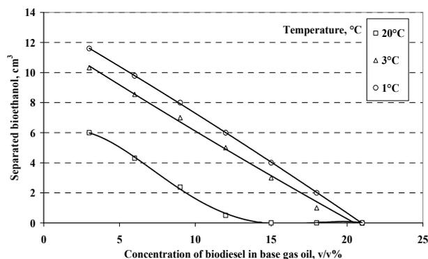
Figure 4: Stability of bioethanol/gas oil emulsions as a function of temperature (2% additive, 15 v/v% bioethanol)
