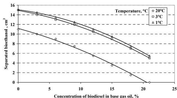
Figure 2: Stability of bioethanol/gas oil emulsions as a function of temperature (without additive, 15 v/v% bioethanol)
