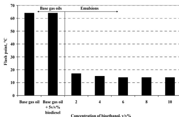
Figure 8: Change of flash point of bioethanol/gas oil and/or biodiesel emulsions as a function of bioethanol content
