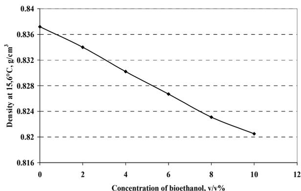
Figure 6: Change of density of bioethanol/gas oil emulsions as a function of bioethanol content
