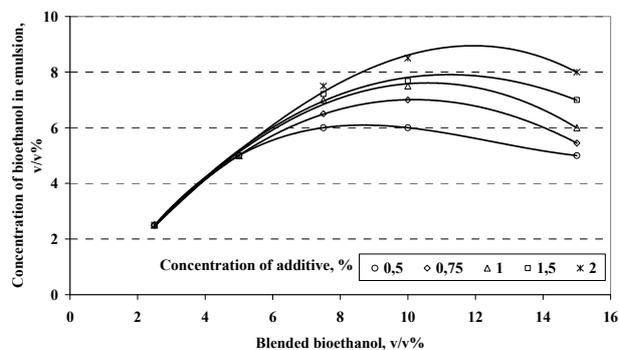
Figure 1: Stability of bioethanol/gas oil emulsions as a function of quantity of additive (temperature: 20 °C)
