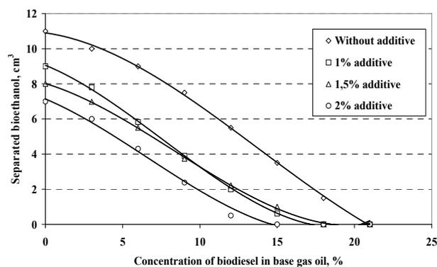
Figure 5: Stability of bioethanol/gas oil emulsions as a function of quantity of additive (temperature: 20 °C, bioethanol content: 15 v/v%)
