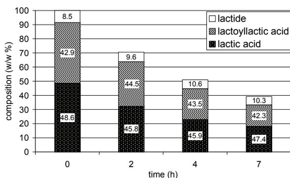
Figure 5: Composition of the LA solution in the reaction mixture vs. reaction time and the ratio of the compounds after certain reaction times (0.7 mmol Cyphos 202 IL, 2 mmol LA, 14 mmol ethanol, 3 w/w% initial water content)
