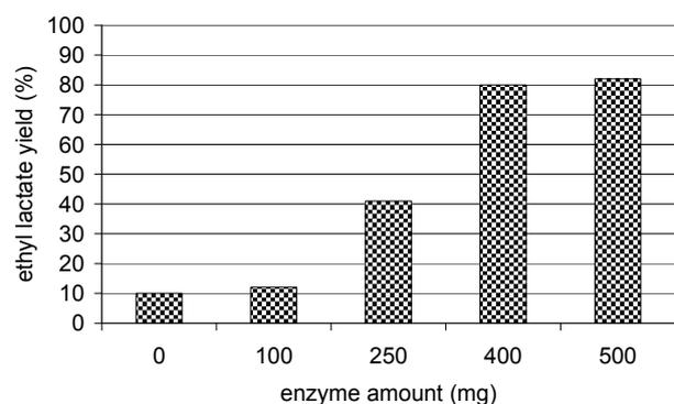
Figure 2: Ethyl lactate yield obtained after 24 h vs. enzyme amount used (LA 1 mmol, ethanol 5 mmol, initial water content 2.5 w/w% diluted with toluene to 5 cm<sup>3</sup>)
