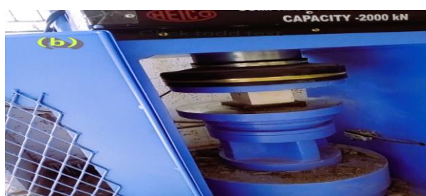
Figure 2: Compressive strength testing: (a) prepared samples - molds and blocks (b) MOS block analyzed by a universal testing machine
