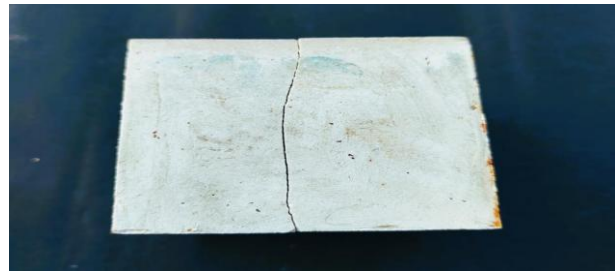
Figure 4: Crack formation in compressive strength testing block of M0 during curing
