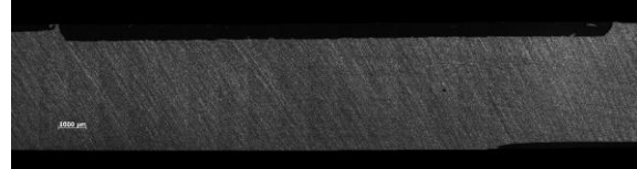
Figure 13: Cross-sectional image of the sample welded by Tool 3 at a feed rate of 125 mm/min
