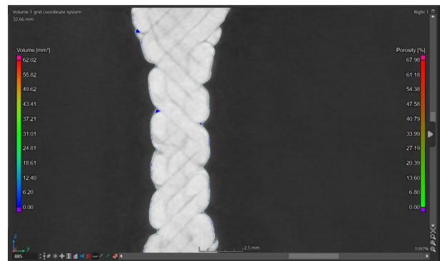
Figure 5: 2D longitudinal section of a 25-45-OI specimen
