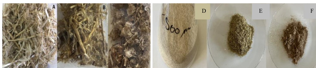
Figure 1: Samples of straw washed with ultrapure water (A), modified with NaOH (B), modified with citric acid (C), ground branches (D), modified with NaOH (E) and modified with citric acid (F)
