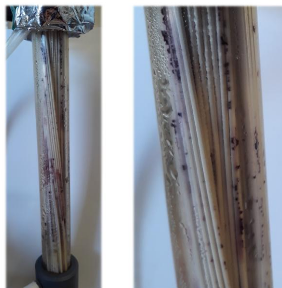
Figure 2: Inconspicuous colonies on the surface of the Pentair X-Flow hollow fibre module
