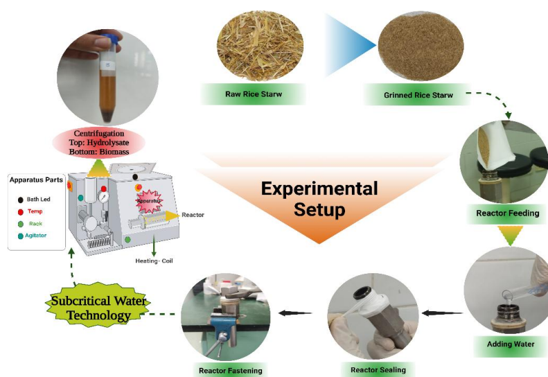
Figure 1: Experimental set-up of rice straw pretreatment using subcritical water technology
