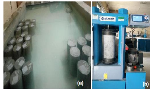
Figure 8: Mechanical testing: (a) Cylindrical specimens (32Φ16), (b) Uniaxial compressive strength tests
