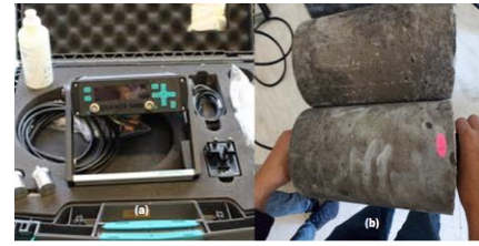
Figure 7: Ultrasonic Pulse Velocity test: (a) UPV device, (b) UPV testing of concrete sample
