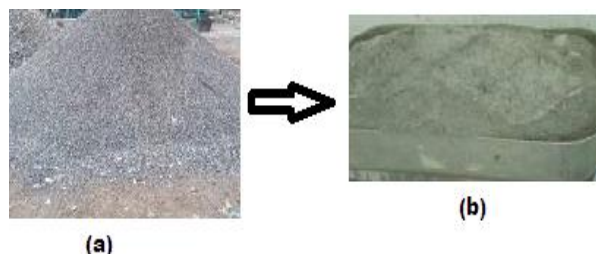
Figure 2: Concrete demolition wastes (CDW): (a) preparation zone, (b) CDW crushed finely
