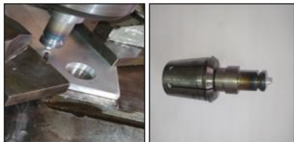
Figure 12: FSW welding tool
