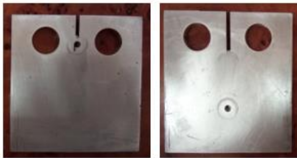
Figure 14: The CT75 specimens after welding
