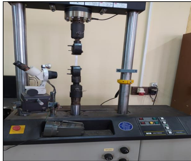
Figure 2: Instron machine used for traction
