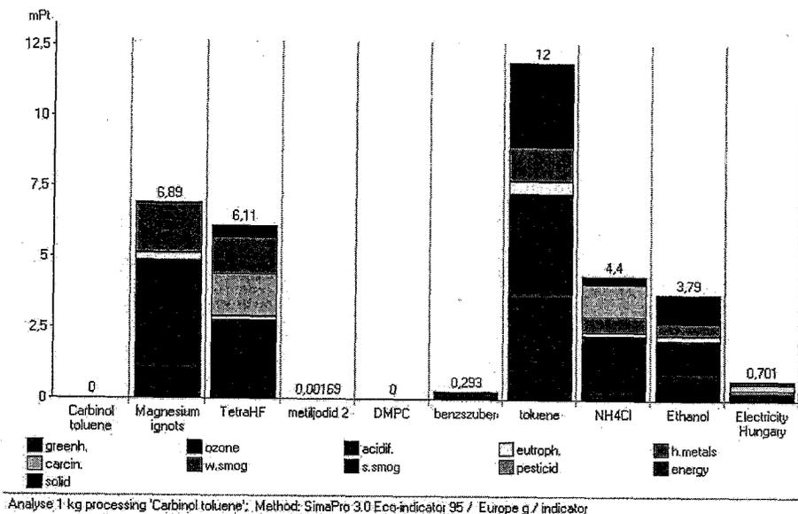
Fig.6 The indicator figure with toluene
