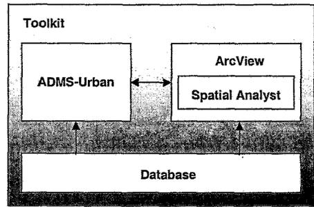
Fig.2 Block diagram of the toolkit
