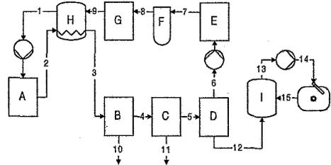
Fig. 6 Dish - mobile (Flows: 1 Fresh water from tank; 2 Waste water from dish - washer; 3,4,5,6,7,8 Circulated water; 9 Reconditioned water in drinking water quality; 10 Oil and fat sludge; 11 Suspended matter; 12 Concentrate; 13, 14, 15 Concentrate is used for preliminary washing of dishes. Processes: A Dish - washer; B Plate precipitator; C Flotation; D Reverse osmosis; E Ion exchanger; F Activated charcoal absorber; G UV sterilisation; H Fresh water tank; I Waste water tank)
