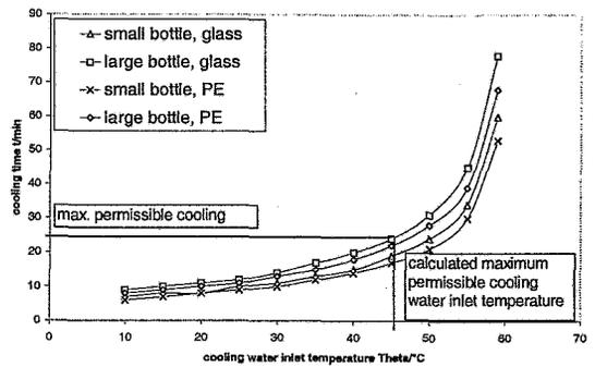
Fig. 5 Result of calculation of cooling time
