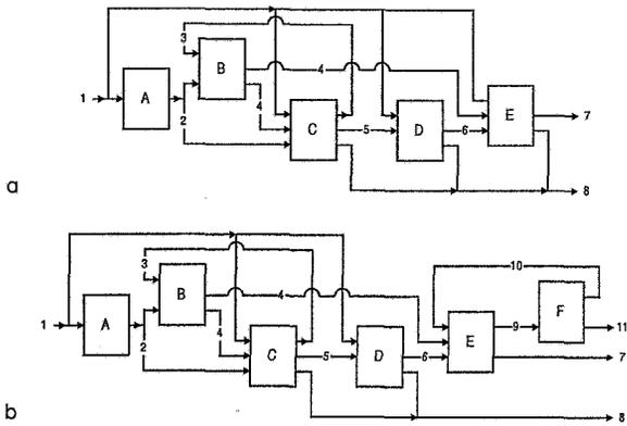
Fig. 4 Flow sheet w/o cooling pond (a/b resp.) Flows: 1 Fresh Water; 2 Demineralised Water; 3 Recirculated Steam; 4 Steam; 5 Distilled Water; 6 Product; 7 Finished Product; 8 Waste Water; 9 To cooling pond (40°C); 10 From cooling pond (30°C); 11 Overflow. Processes: A Demineralisation; B Steam Boiler; C Distiller; D Mixing Process; E Autoclave; F Cooling pond
