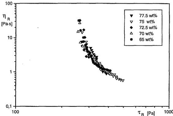
Fig.6 Reduced viscosity ( $\eta_R$ ) vs. reduced shear stress master curve for the alumina slips investigated.
