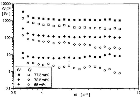
Fig.7 Storage ( $G'$ ) and loss ( $G''$ ) moduli variation with angular velocity ( $\omega$ ) for some of the alumina suspensions studied (0.7 rad of constant strain).
