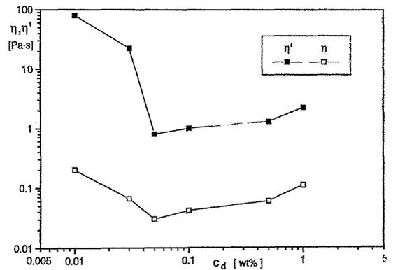
Fig.9 Apparent ( $\eta$ ) and dynamic ( $\eta'$ ) viscosity vs. deflocculant concentration ( $\dot{\gamma} = 200 \text{ s}^{-1}$ ;  $\omega = 2 \text{ s}^{-1}$ ).
