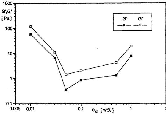
Fig.10 Storage ( $G'$ ) and loss ( $G''$ ) moduli vs. deflocculant concentration ( $\omega = 2s^{-1}$ ).
