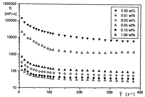
Fig.8 Apparent viscosity ( $\eta$ ) vs. shear rate ( $\dot{\gamma}$ ) flow curves for the 77.5 wt% alumina + sodium polyphosphate suspensions studied.
