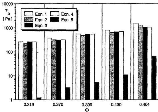
Fig.2 Yield stress ( $\tau_0$ ) variation with solid volume fraction ( $\Phi$ ) for the alumina suspensions studied.
