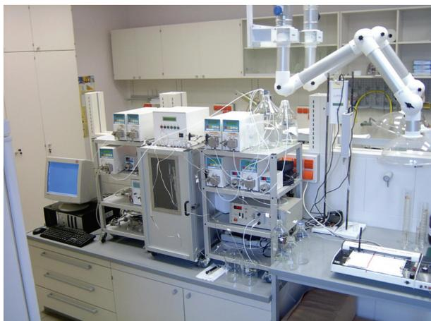
Fig. 4.: KNAUER CSEP 9116 SMB unit assembled for quasi-continuous process
