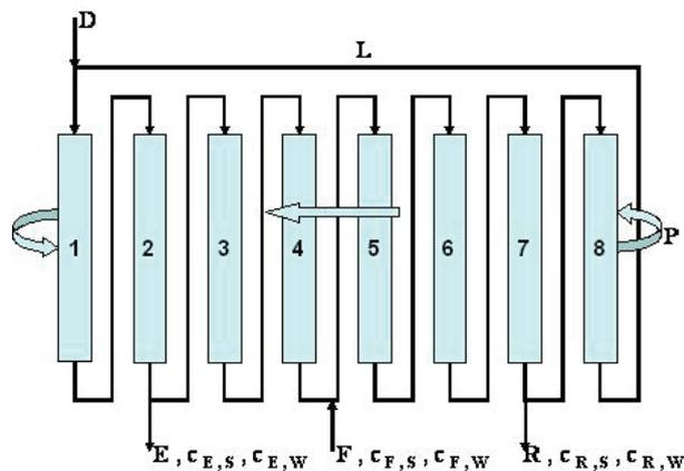
Fig. 2.: One of the applied practical solutions of the Simulated Moving Bed
