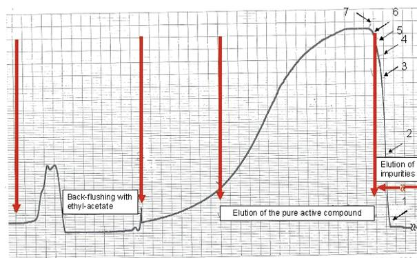
Fig. 5.: Chromatogram of the preliminary elution experiment
