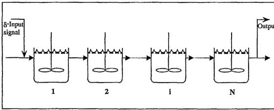
Fig.1 Schematic of MFRs in series
