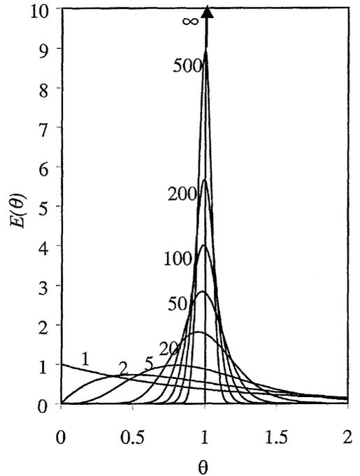
Fig.2 RTD curves for MFRs in series
