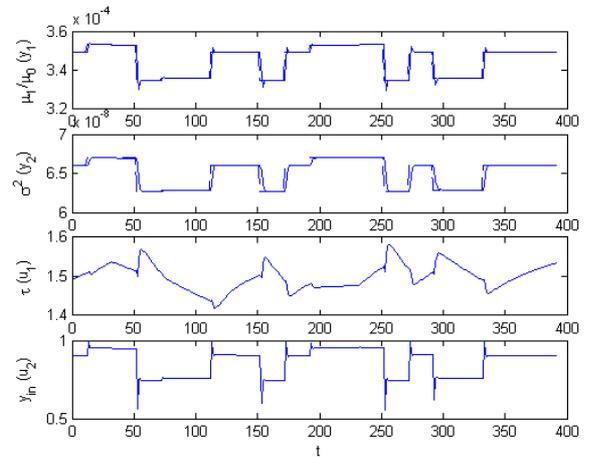
Fig.4. Performance of the MPC of the continuous isothermal MSMR crystallizer
