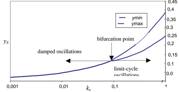
Fig. 3: Bifurcation diagram  $k_e$ - $y_s$  of the crystallizer
