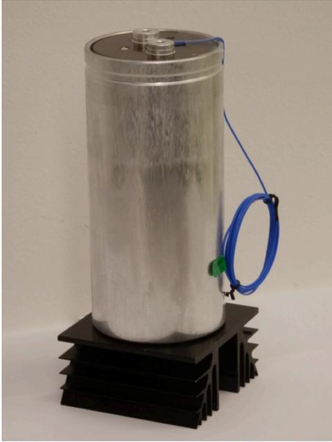
Figure 7: Core temperature measurement of a capacitor
