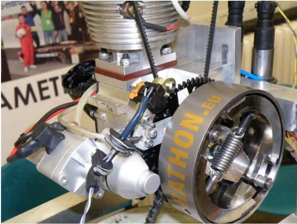
Figure 6: Setup for measuring the instantaneous torque
