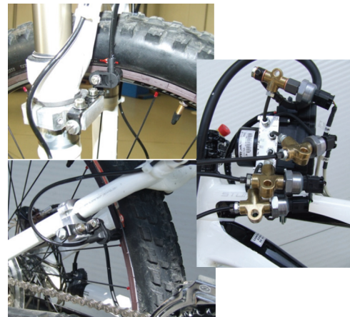
Figure 4: Speed and pressure sensors on the bicycle
