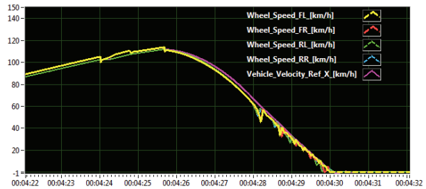
Figure 18: The vehicle velocity (km/h) and wheel speeds (km/h) with the ABS ECU (emergency braking from 115 km/h)
