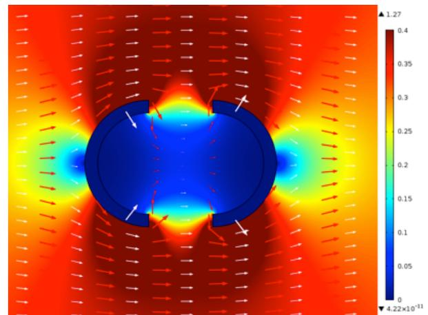
Figure 6: Simulation of shielding for shell geometry
